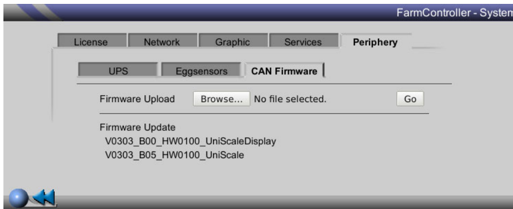
Figure 4-29: CAN modules: uploading new firmware
